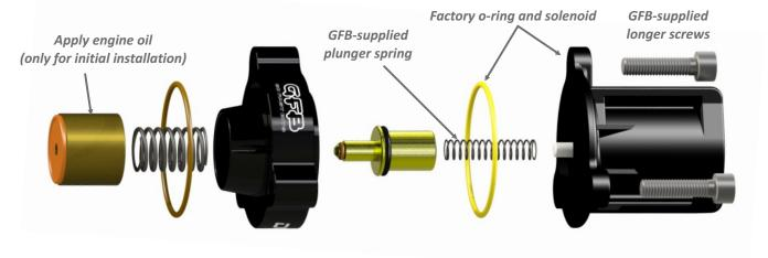
During assembly, check that the piston slides freely in the body without sticking or binding. It is a very close fit and can sometimes be difficult to get started into the bore, but once in it should move without needing to be forced. Apply some engine oil onto the piston during assembly. It is **NOT necessary to regularly lubricate the piston after assembly.**
