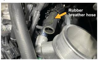
5) Using a 10mm socket, remove the two bolts that hold the metal intake to the turbo. Remove it from the turbo flange and leave it supported by the two coolant hoses that are still attached:
